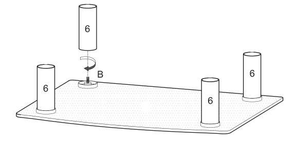
Screw cylinders (6) onto short rods (B).
